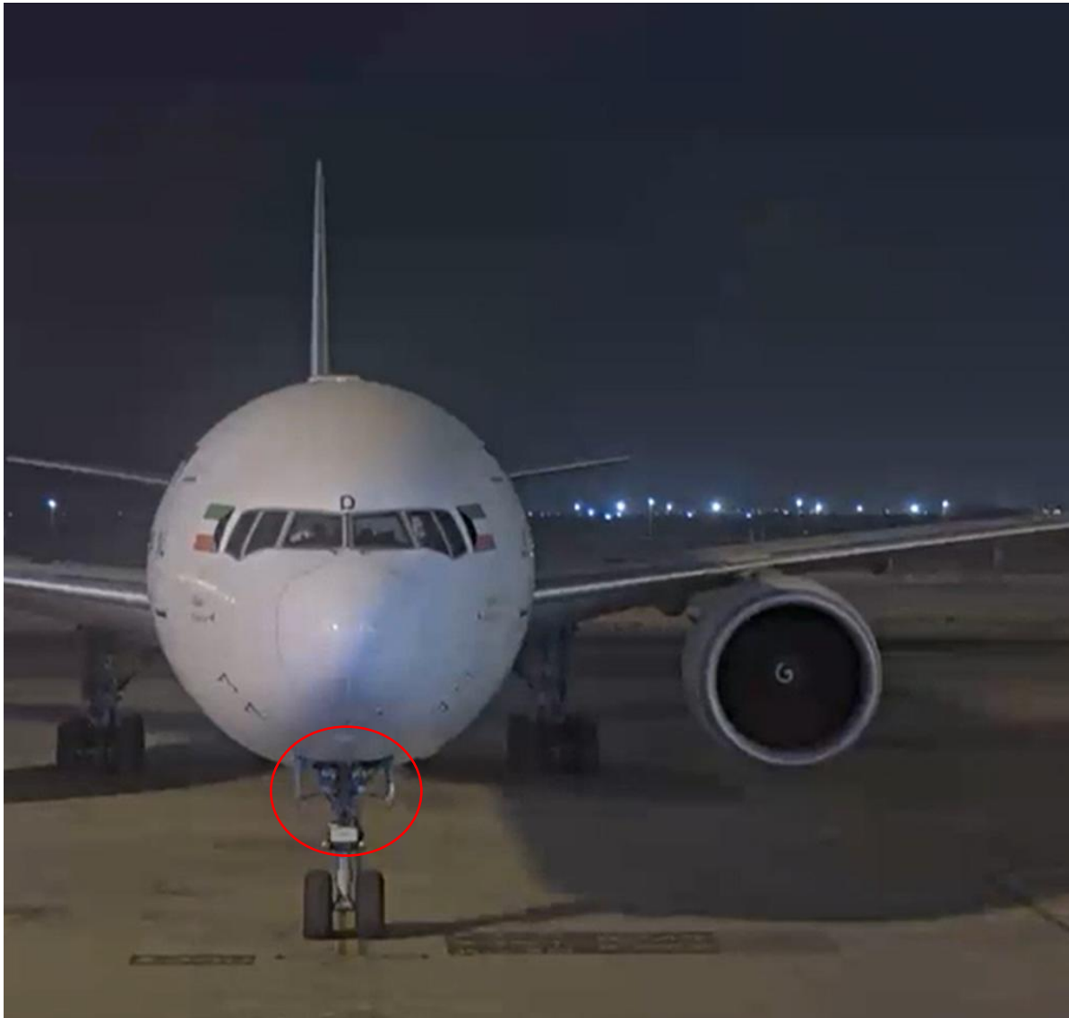
Figure 3: No Lights Visible on The Nose Landing Gear
