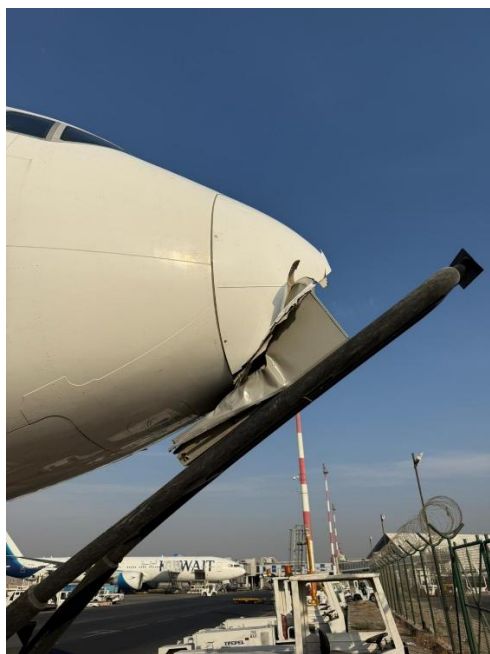
Figure 7: Nose Striking the Stand Pole
