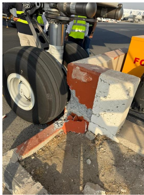
Figure 6: Wheel Hitting the Pole Base
