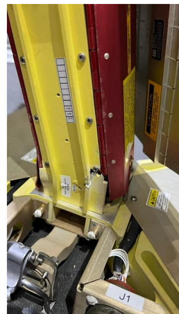
Figure 10: Weather Radar Base Cracked
